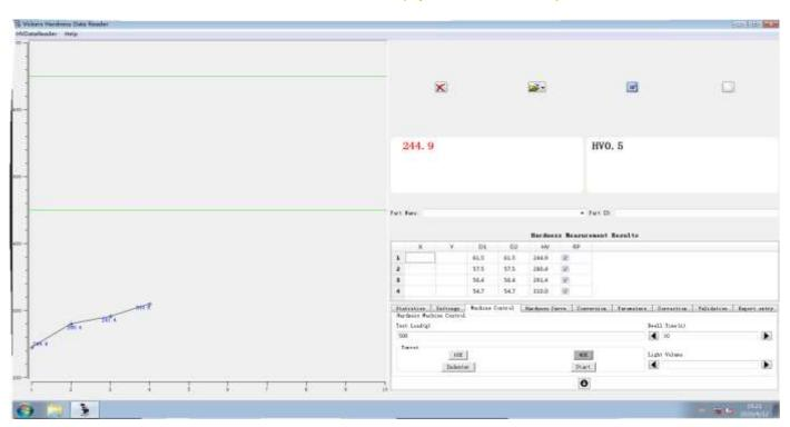
Software can control the machine turret and generate test report including hardness value curve. Software install on the computer, connect with hardness tester through RS232 port. All the testing result can save to computer and generate test report in word format.
